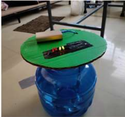
Fig- 2.4: Small model of overhead water tank with all sensors embedded
